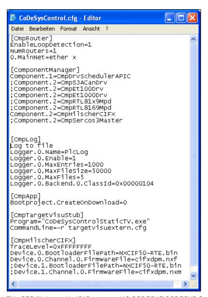
This CFG file located in "C:\Programme\3S CODESYS\CODESYS Control RTE3\" configures one CIFX 50-DP(M/S) card for use with a RTE runtime system.
